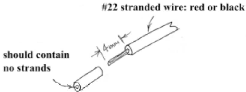
**Figure 3: Stripping wires**
